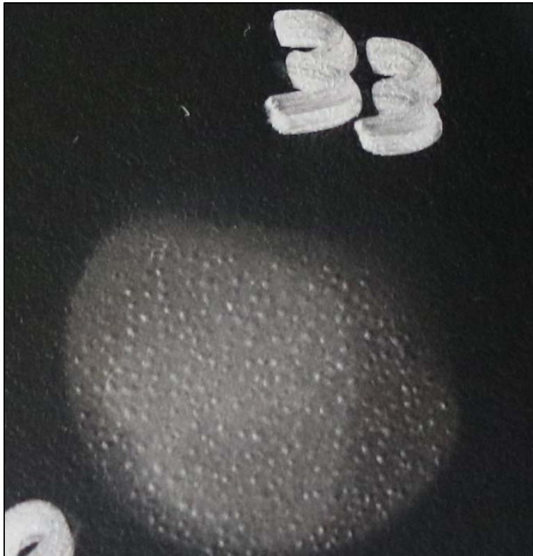
Chemical spot test #33, Nitric Acid (70%), Rating 3, Surface swelling
