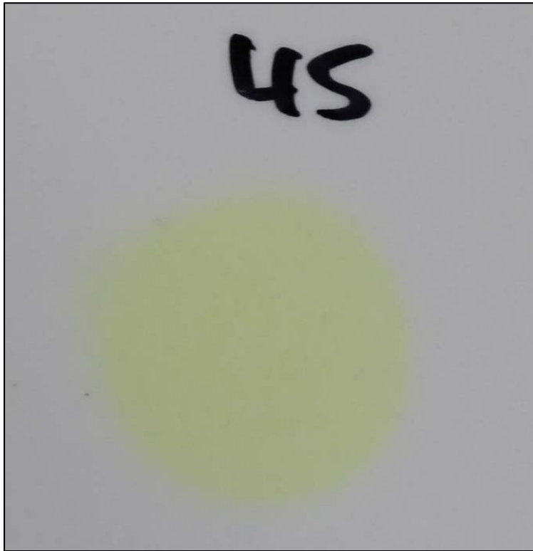
Chemical spot test #45, Sulfuric Acid (77%) and Nitric Acid (70%), equal parts, Rating 2, Color change
