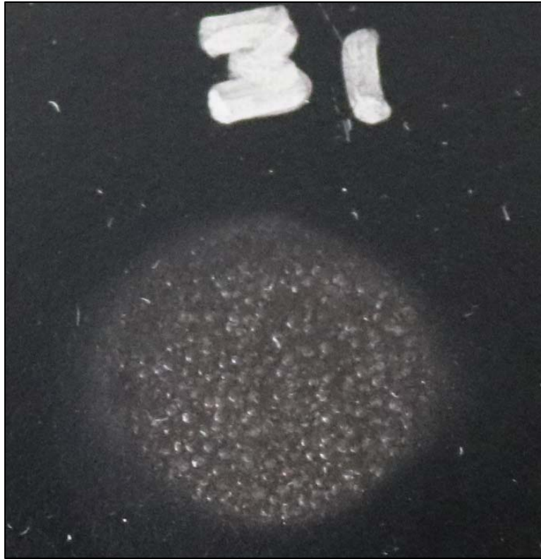
Chemical spot test #31, Nitric Acid (20%), Rating 3, Surface swelling
