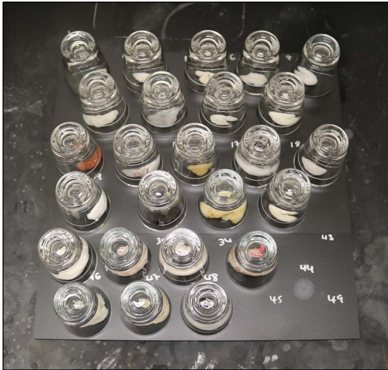
Representative Chemical Spot Test Volatile Chemical Set-up
